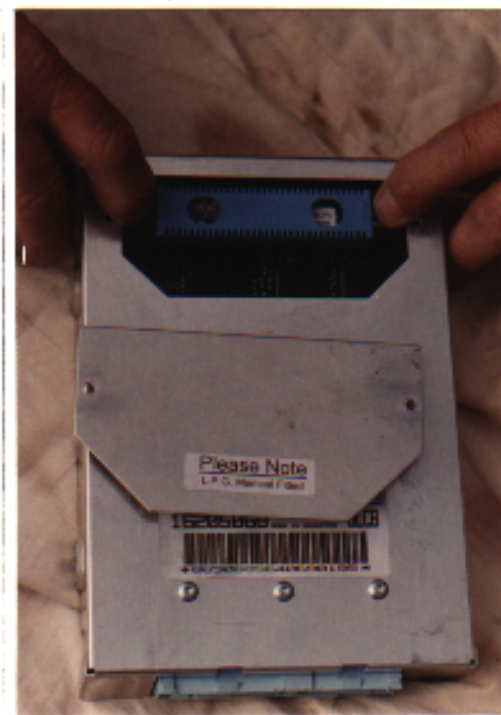
Fig. 6 Fitting a Memcal
