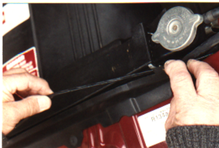
Fig. 12 Engine Bay Loom Being Fitted Under Radiator Trim
