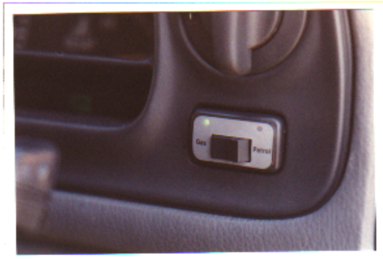
Fig. 1 Apexus PS105 LPG/Petrol mode switch
